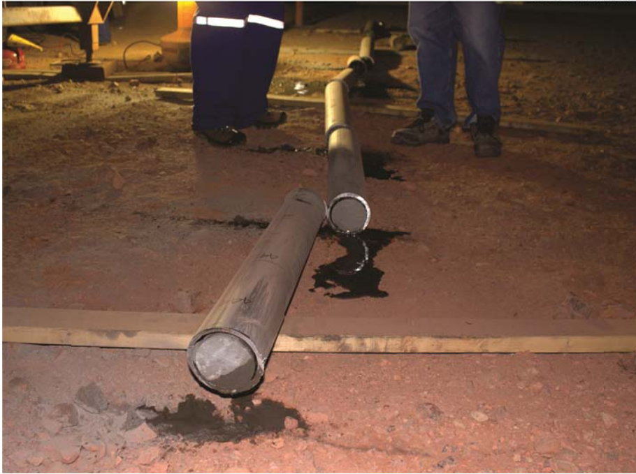
Figure 7. Cut core barrel sections from 33-14R prior to transport to Weatherford Core Labs (March 2013).
