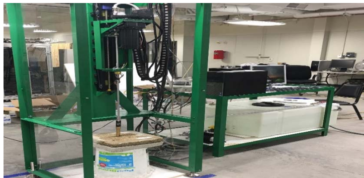
Figure 1: Lab-scale Automated drill Rig tested drilling a vertical Hole
