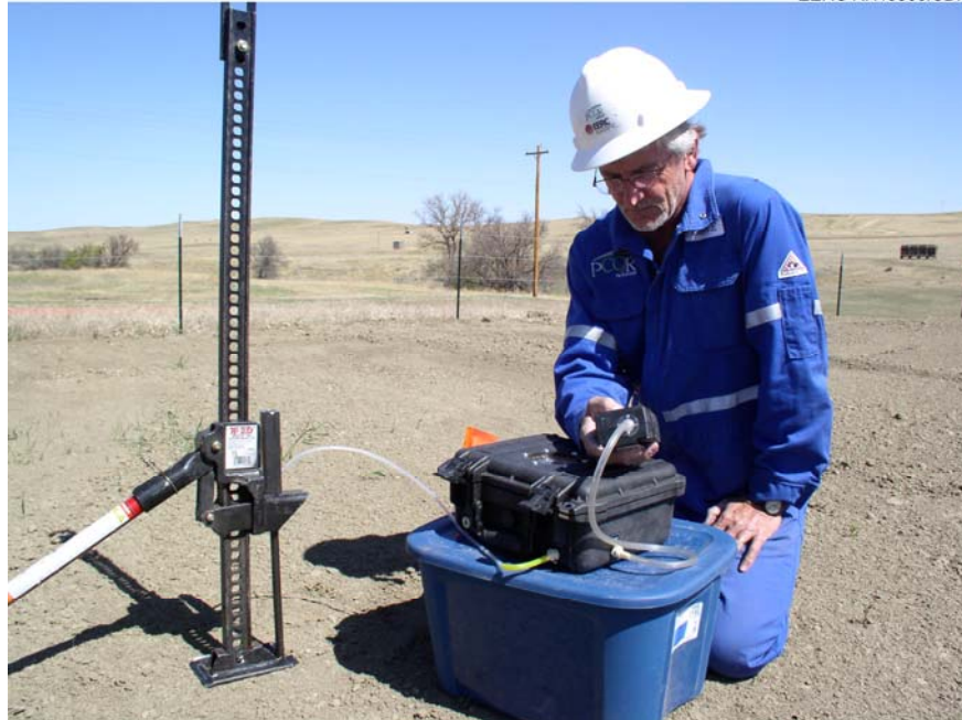
Figure 3. Collecting soil gas samples from a production pad in the Bell Creek Field.
