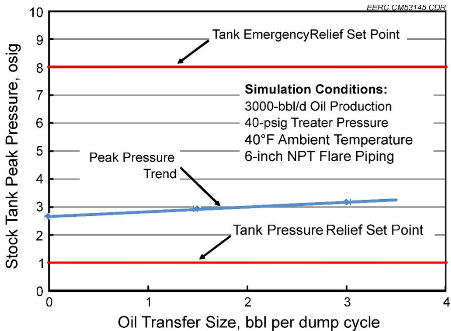
Figure 6. Parametric evaluation results for peak tank pressures. Zero oil transfer size corresponds to a continuous fill scenario.
