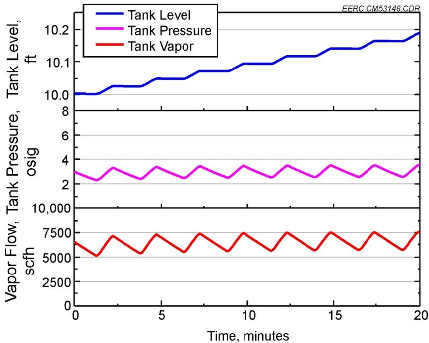
Figure 5. Dynamic modeling of a pulse filling operation. Conditions include 3-bbl oil transfer per dump cycle, 3000-bbl/day oil throughput, 40-psig separator pressure, 40°F ambient temperature, and 6-inch NPT flare piping.
