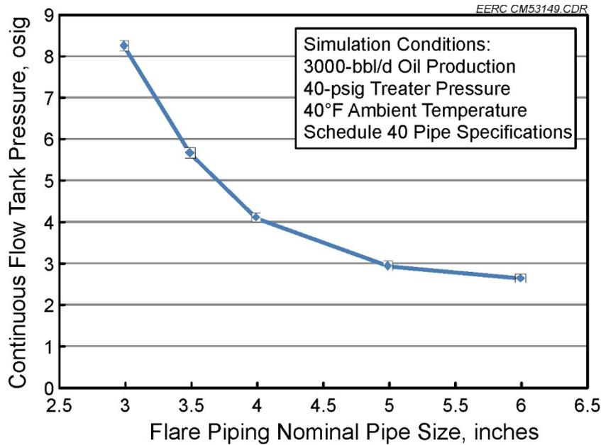
Figure 7. Sensitivity of tank pressure to flare pipe size.
