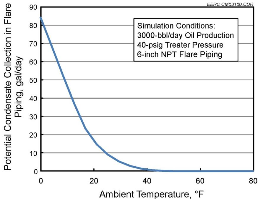
Figure 8. Estimated rates of tank vapor condensate formation.
