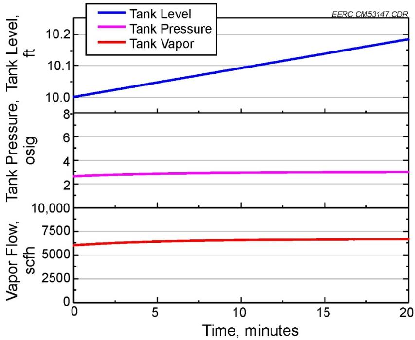
Figure 4. Dynamic modeling of a continuous tank-filling operation. Conditions include 3000-bbl/day oil throughput, 40-psig separator pressure, 40°F ambient temperature, and 6-inch NPT flare piping.
