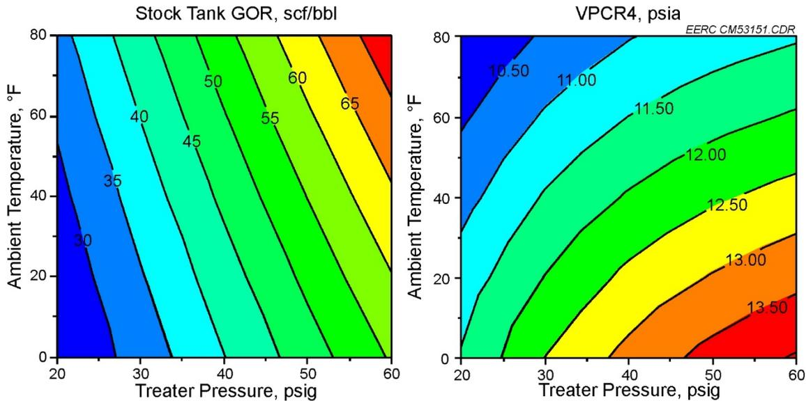
Figure 3. Modeling results for tank vapor emission factor and the produced oil’s vapor pressure.
