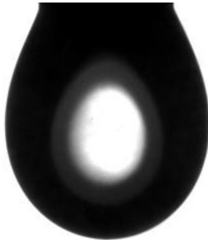
Figure 11. Image of Distilled Water Surface Tension Measurement using IFT-10 Pendant Drop Tension Cell
