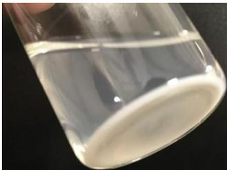
**Figure 32.** Aggregation of silica nanoparticles solution of 0.5wt% concentration at Day 4 at 80°C
