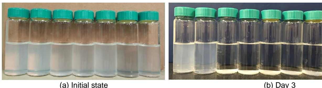
(a) Initial state (b) Day 3 Figure 18. The effects of salinity on the stability of silica nanoparticles (20°C)
