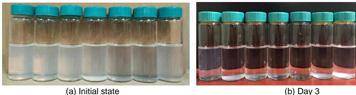
(a) Initial state (b) Day 3 Figure 17. The effects of salinity on the stability of silica nanoparticles (80°C)
