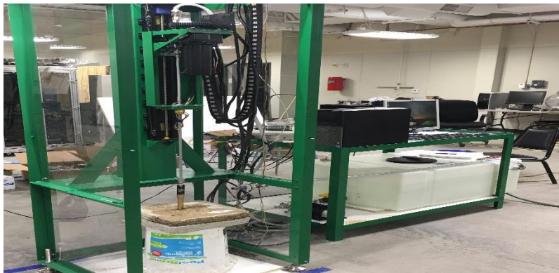
Figure 3: Lab-scale Automated drill Rig initially used for drilling a vertical
