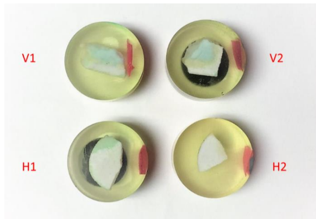
Figure 3 3D printed rock fragments for nanoindentation experiments. 'V' represents vertical, and 'H' denotes horizontal.
