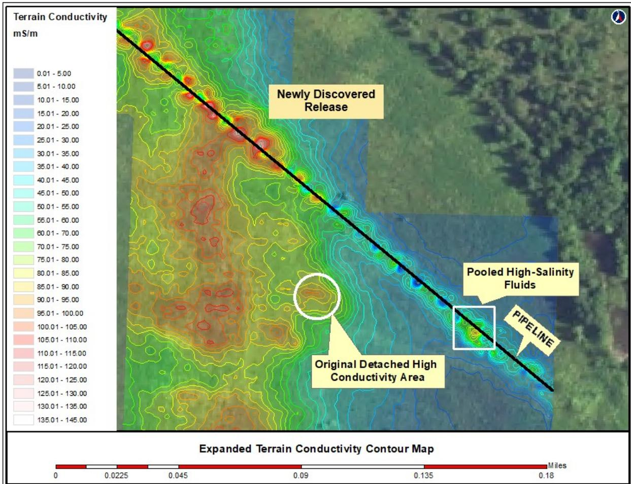
The expanded EM-31 Survey revealed a large plume of highly conductive material in the subsurface further along the pipeline to the northwest. The data indicated a breach of the flowline that had been undetected until the EM-31 Survey was implemented.
