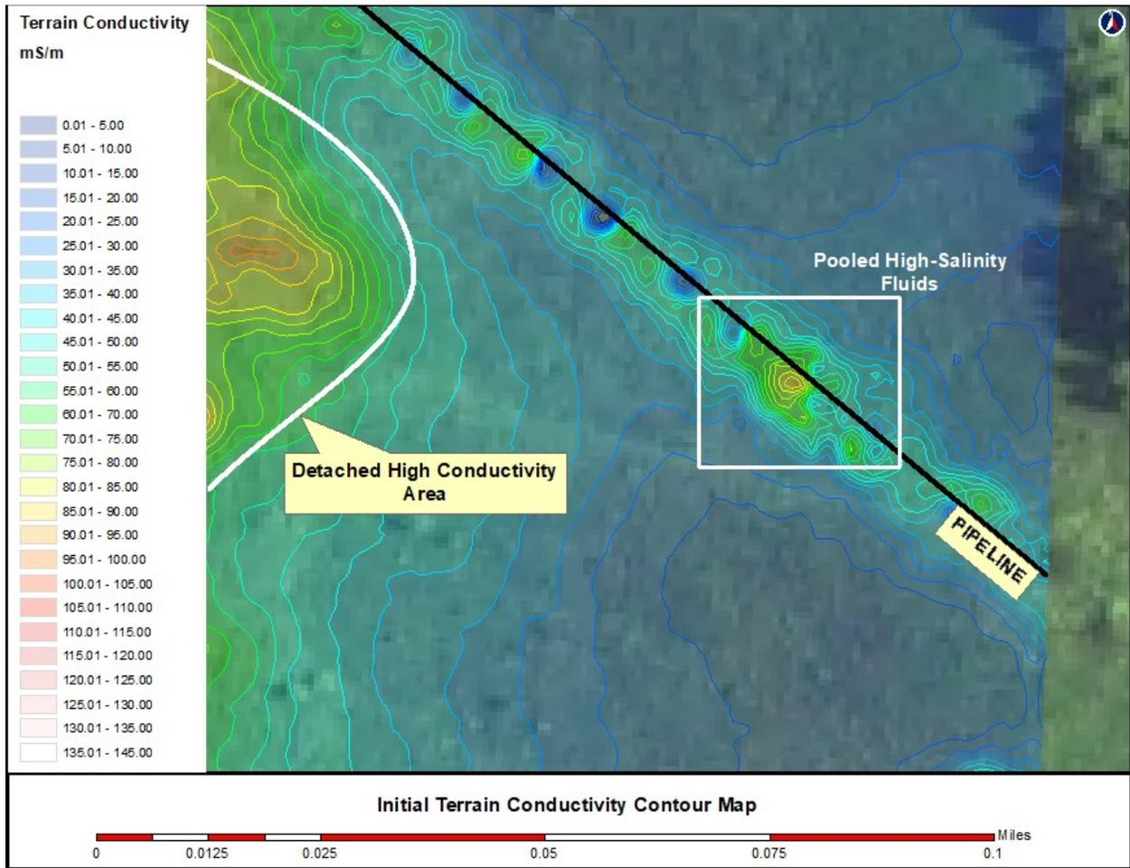
Results of the EM Survey clearly imaged the straight, linear conductivity signature of the underground flowline, and the area of high conductivity at the location of the pooled high-salinity liquids.
