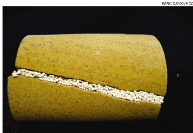
Figure 4. Image depicting a proppant pack placed in core (Bremer and others, 2010).
