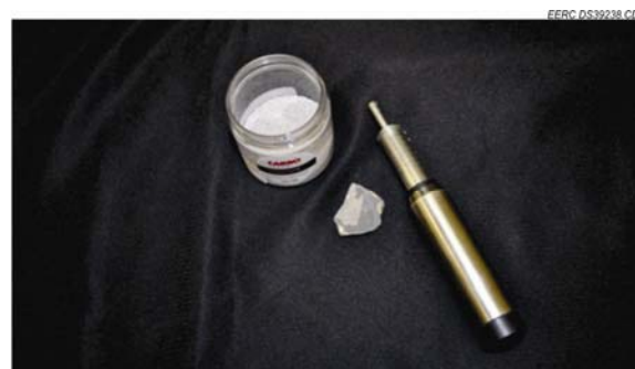
Figure 2. Penetrometer for embedding proppant.
