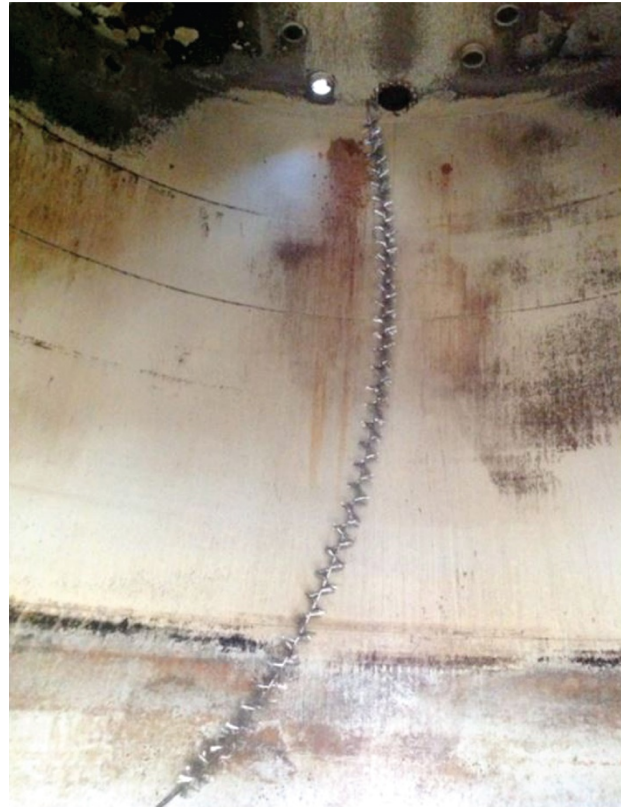
Figure 8. Example of in-tank static dissipater (source: Lightning Master Corporation).
