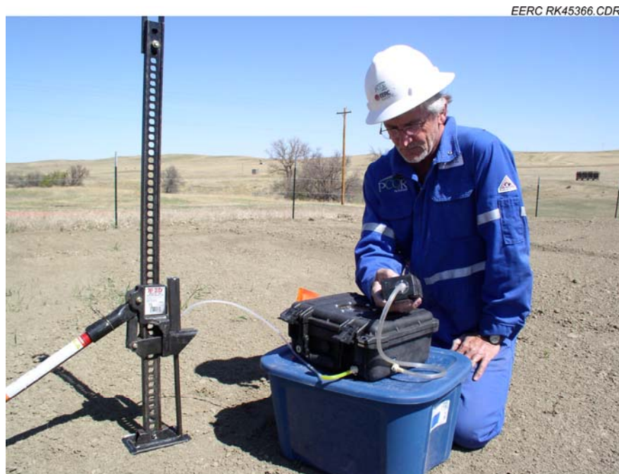
Figure 3. Collecting soil gas samples from a production pad in the Bell Creek Field.
