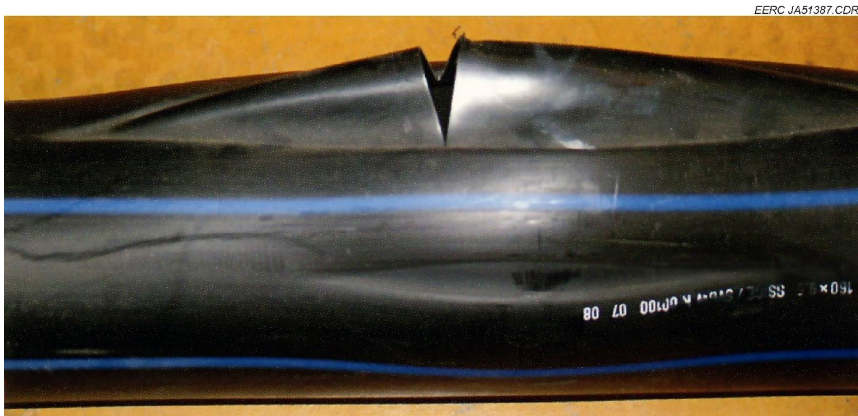
Figure 27. An example of a pipe that failed through slow crack growth (Farshad, 2006).
