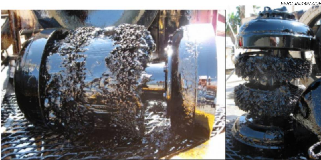
Figure 45. Brush pig after emerging from Cleaning Run 2.
