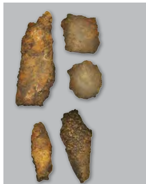
Figure 2. Scale deposits collected from the outside of the sample CS2 casing.
