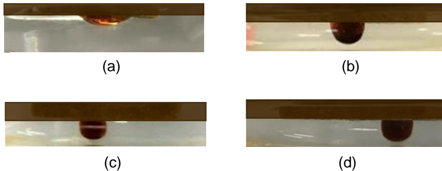
Figure 3. Oil droplet at oil/aqueous/rock interface. (a) 2,000 mg/L KCl brine. (b) 1000 mg/L MERPOL HCS surfactant. (c) 1,000 mg/L MERPOL HCS surfactant + 2,000 mg/L LUDOX SM-
