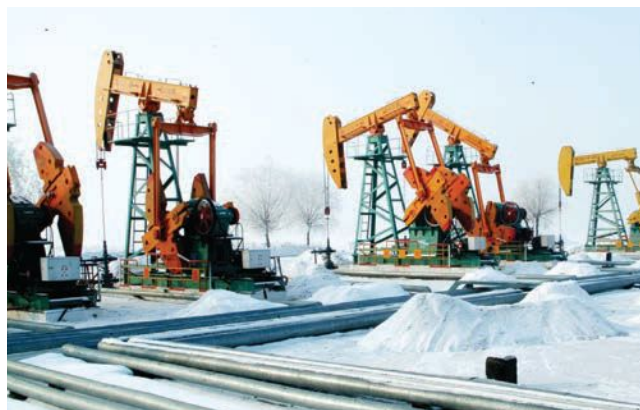
Pipes throughout the Daqing field, located in the frigid northeast corner of China, are needed for the polymer-enhanced water injection and production systems used to enhance production. Photo: Jiamaomimi, depositphotos.com.
