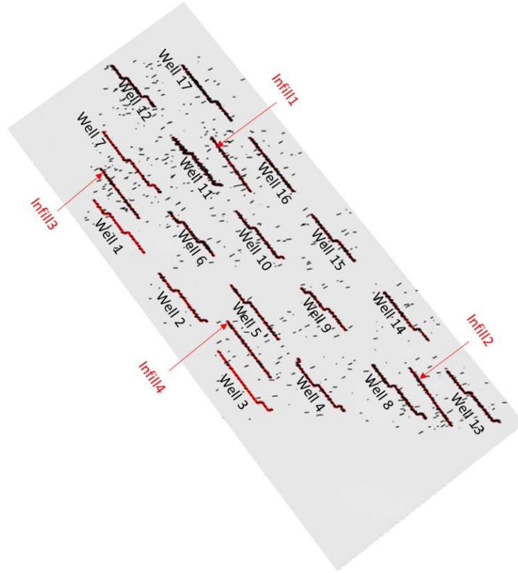
Figure C-19. Distribution of wells and natural fractures for the model with four infill wells.
