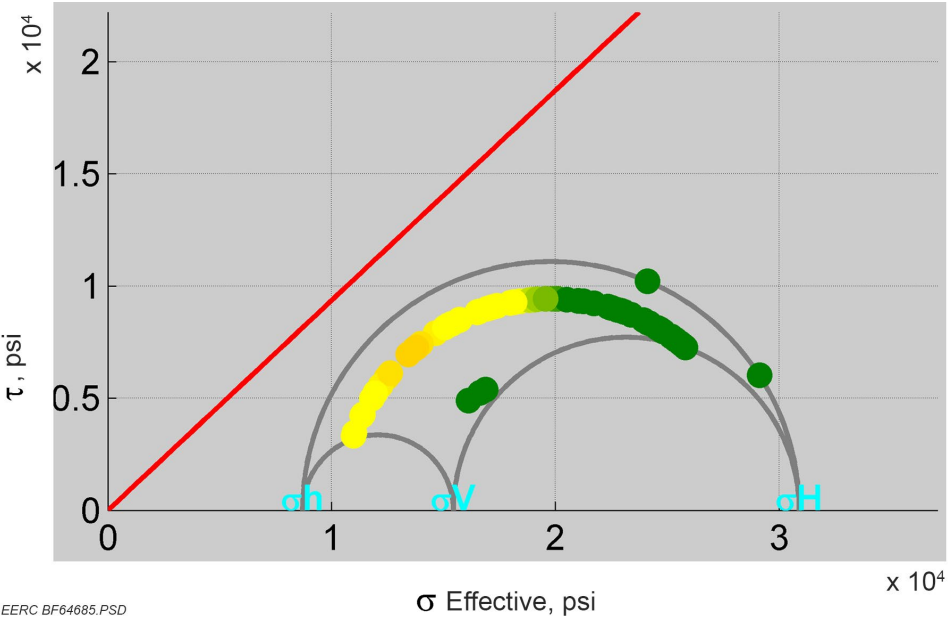
Figure 34. Greater Green River deterministic Mohr–Coulomb analysis of faults. The red line on the left indicates the edge of the fault failure envelope. Green dots indicate faults that are more stable vs. yellow and orange dots that are less stable.
