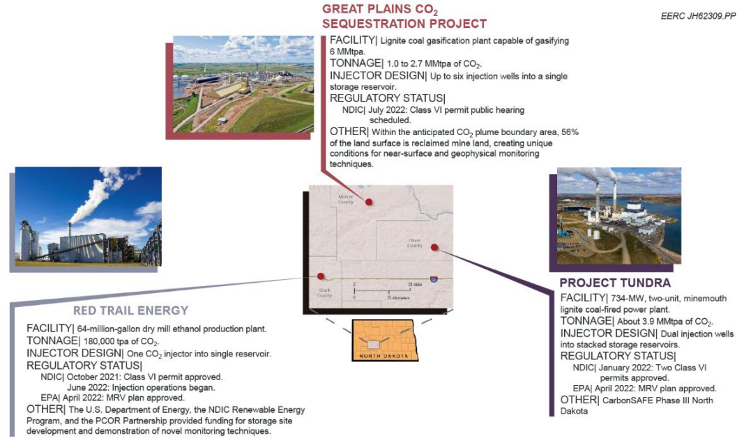
Figure 2-12. Summaries of the RTE CCS Project, Project Tundra, and the Great Plains CO 2 Sequestration Project (modified after Hamling and others, 2022).
