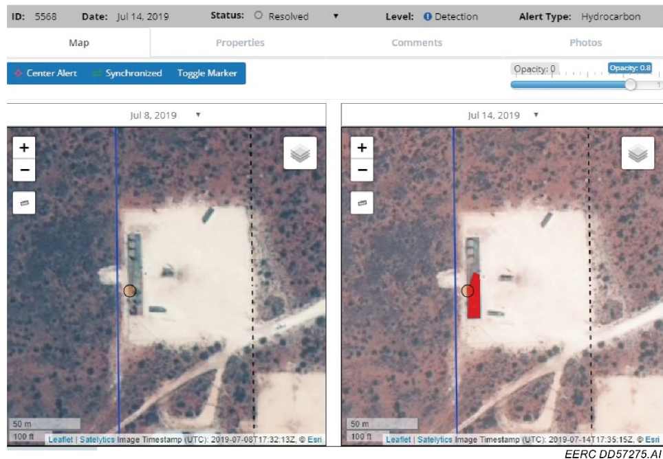
Figure 8. Confirmed New Mexico hydrocarbon leak at a tank battery, nonmember asset (Alert 5568).
