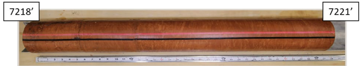
Spearfish FM, Belfield Member (siltstone). This directly underlies the Pine Member Salt
