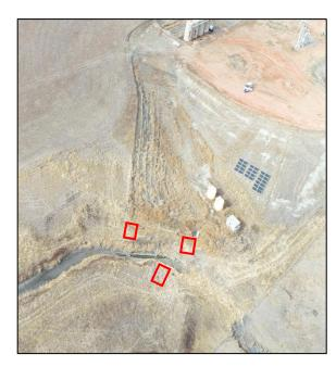
**Oasis Project** – install 2" sand packed wells and work with different pumps and pump rates to overcome ion mounding at the electrode. Three cells (27 wells) will be installed and operated for two seasons. Groundwater and soil data will be collected and reported to demonstrate success
