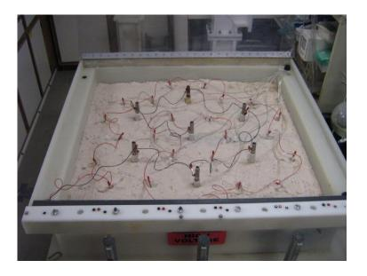
**NDSU** – prepare a bench scale treatment cell where industry can send impacted soil samples. The samples can be tested and modeled to develop a treatment design.
