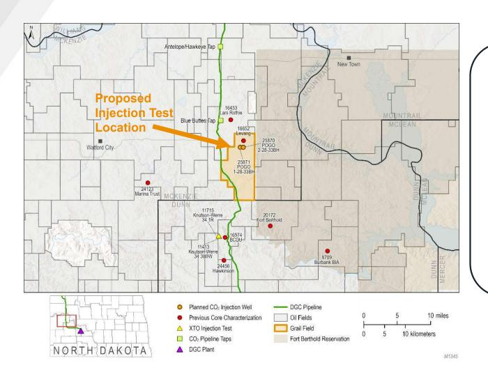
A Chord operated well in a Bakken DSU in the Grail Field, McKenzie County, will serve as the EOR field test location.
